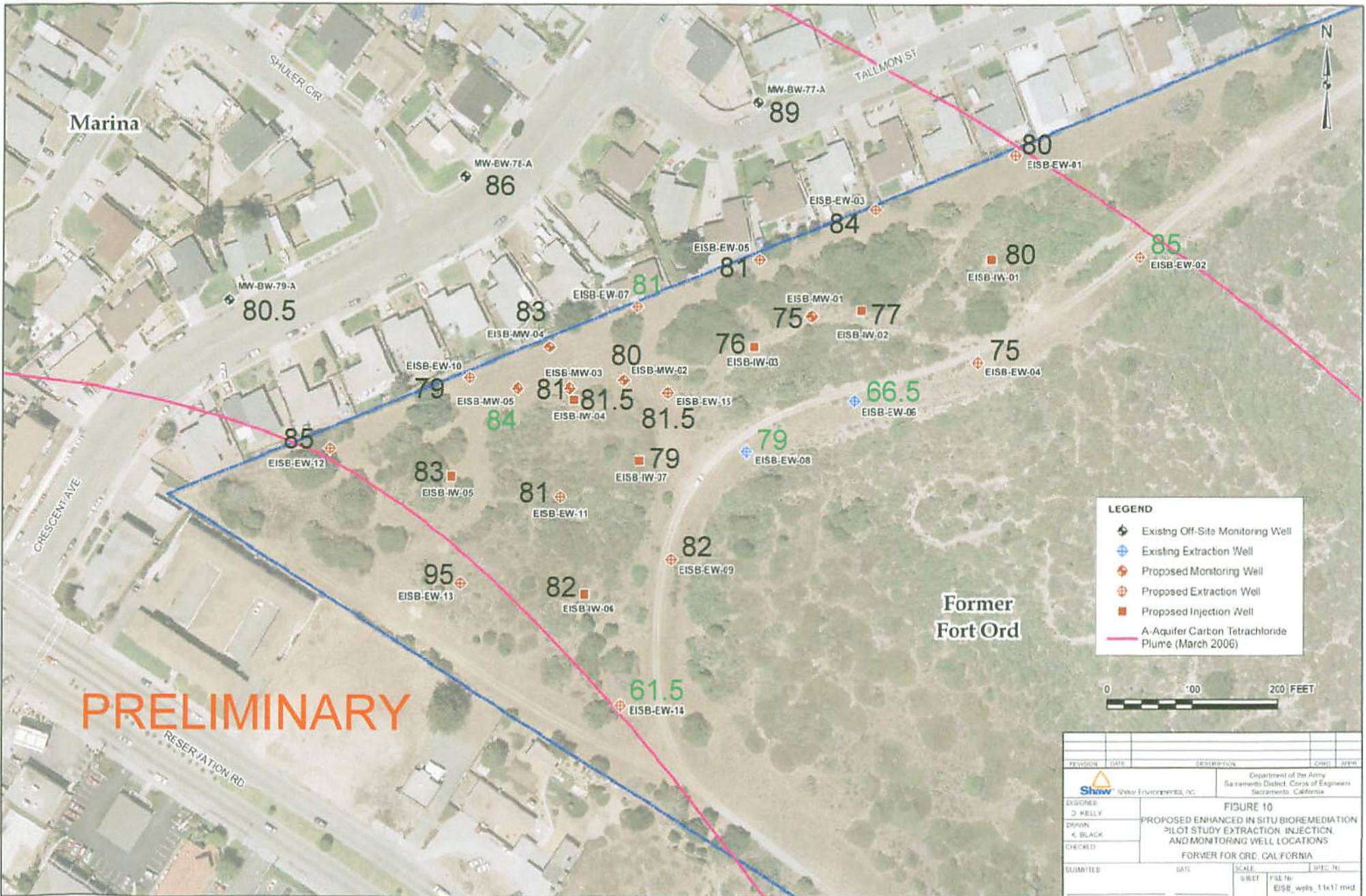
Approximate Depth to Top of Fort Ord – Salinas Valley Aquitard (depths in feet below ground surface) (green – from continuous core samples)
