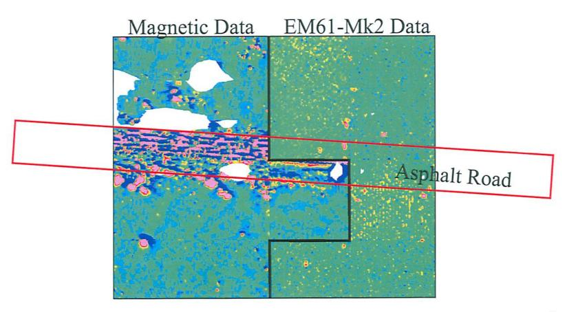
Does the asphalt found at the Former Fort Ord affect the ability of the EM61-Mk2 to detect subsurface metal items?
