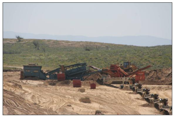
Photograph 7-4 — Conveyer belts in the background deposited debris into containers for transportation to sorting areas, while the series of conveyers in the lower right of the photograph carried sifted dirt to a storage area until it was used to restore the original contours of the scraped area.
