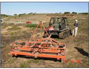
Photographs 6-1 and 6-2 — Individual and towed-array systems were used for the EM61-MK2 surveys on Ranges 43-48.
