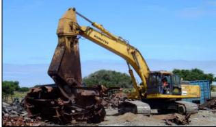
Photographs 4-7 and 4-8 — The range targets were cut by torch or a large mechanical shear.
