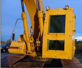
Photographs 7-2 and 7-3 — The armoring of heavy equipment such as the tracked dump truck (left) and excavator (right) entailed reinforcing the operator cab with steel and with Lexan<sup>®</sup> or bullet-resistant glass.
