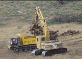
Photographs 4-5 and 4-6 — UXO technicians inspect a range target (left) before it is picked up by an armored excavator and loaded into an armored dump truck (right).
