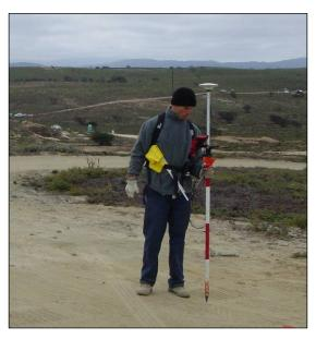
Photograph 6-3 — A Leica GPS receiver attached to the digital survey instruments accurately recorded the locations of data collection points. This enabled anomalous areas to be found easily with the GPS later for verification and excavation.
