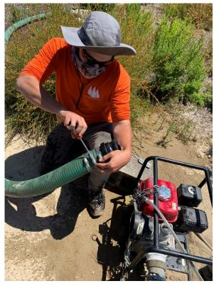
Photo 15: Burleson biologist repairing leak in output hose
